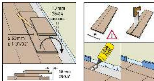
7. Before attaching the **skirting boards**, first use a Stanley knife or cutter to trim excess membrane so it will not protrude above them. It is best to cut the skirting boards to size with a miter saw. (refer to the diagram on the right)
